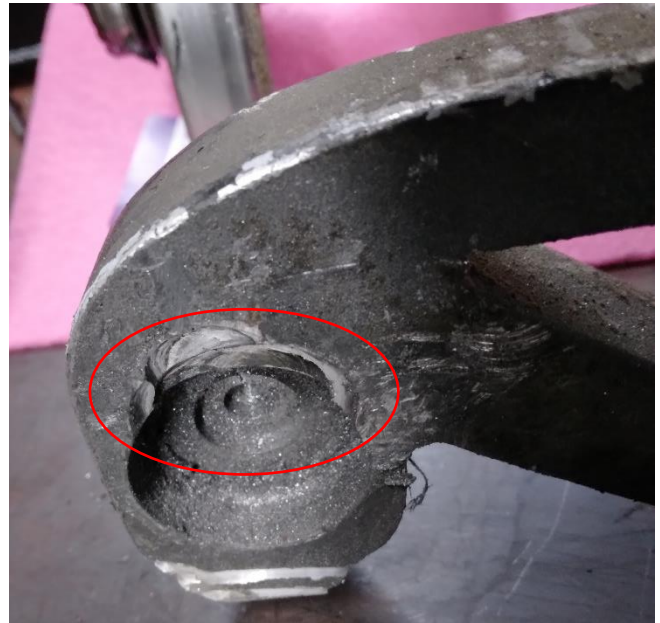
Failed bearing allowed the axle run against the top of the journal box.
