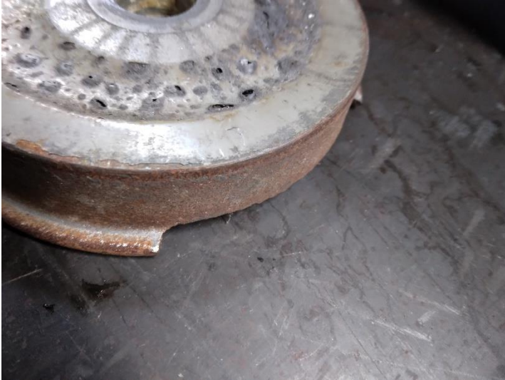
Iron wheel with a broken flange.
